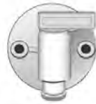
Exterior fresh water drain
